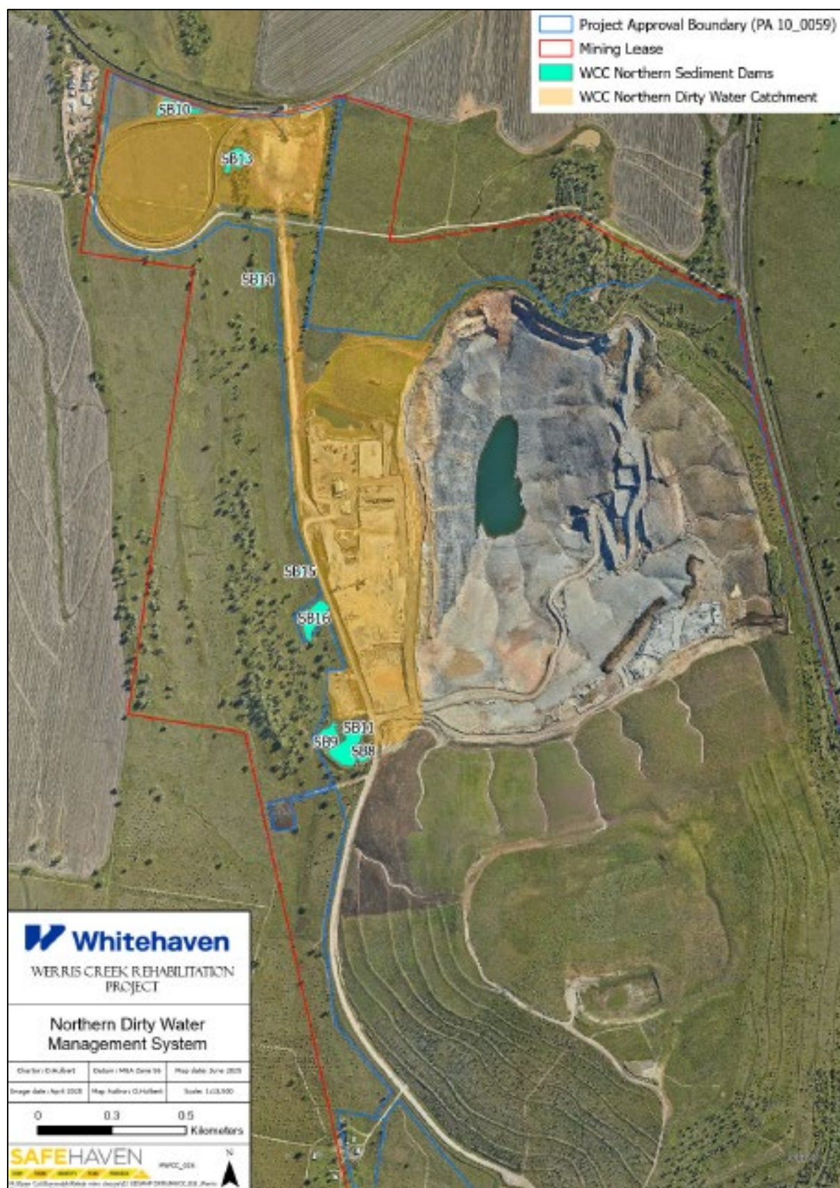
Figure 16 - Middle and Northern Dirty Water Management Systems
