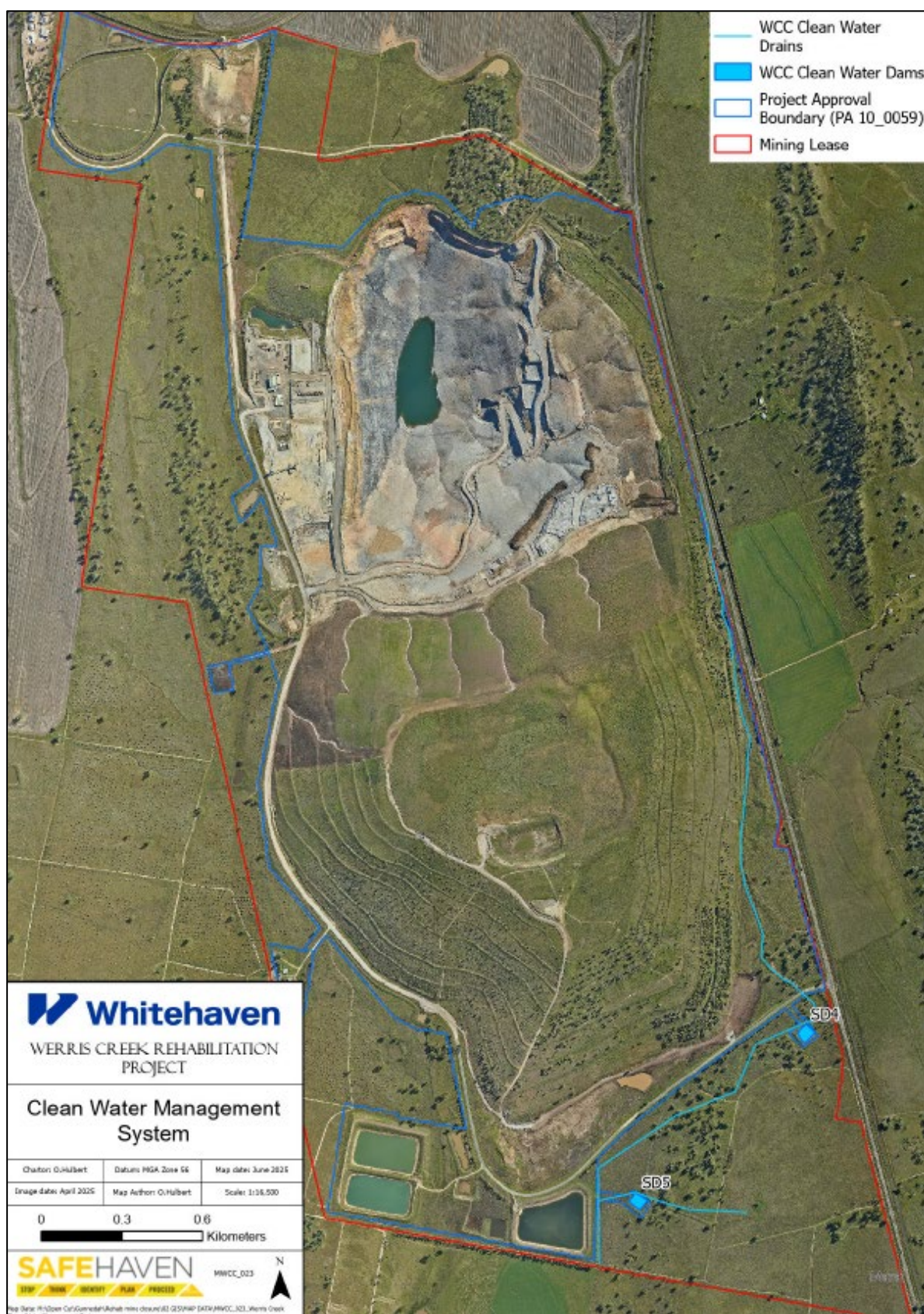
Figure 18 - WCC Clean Water Management System
