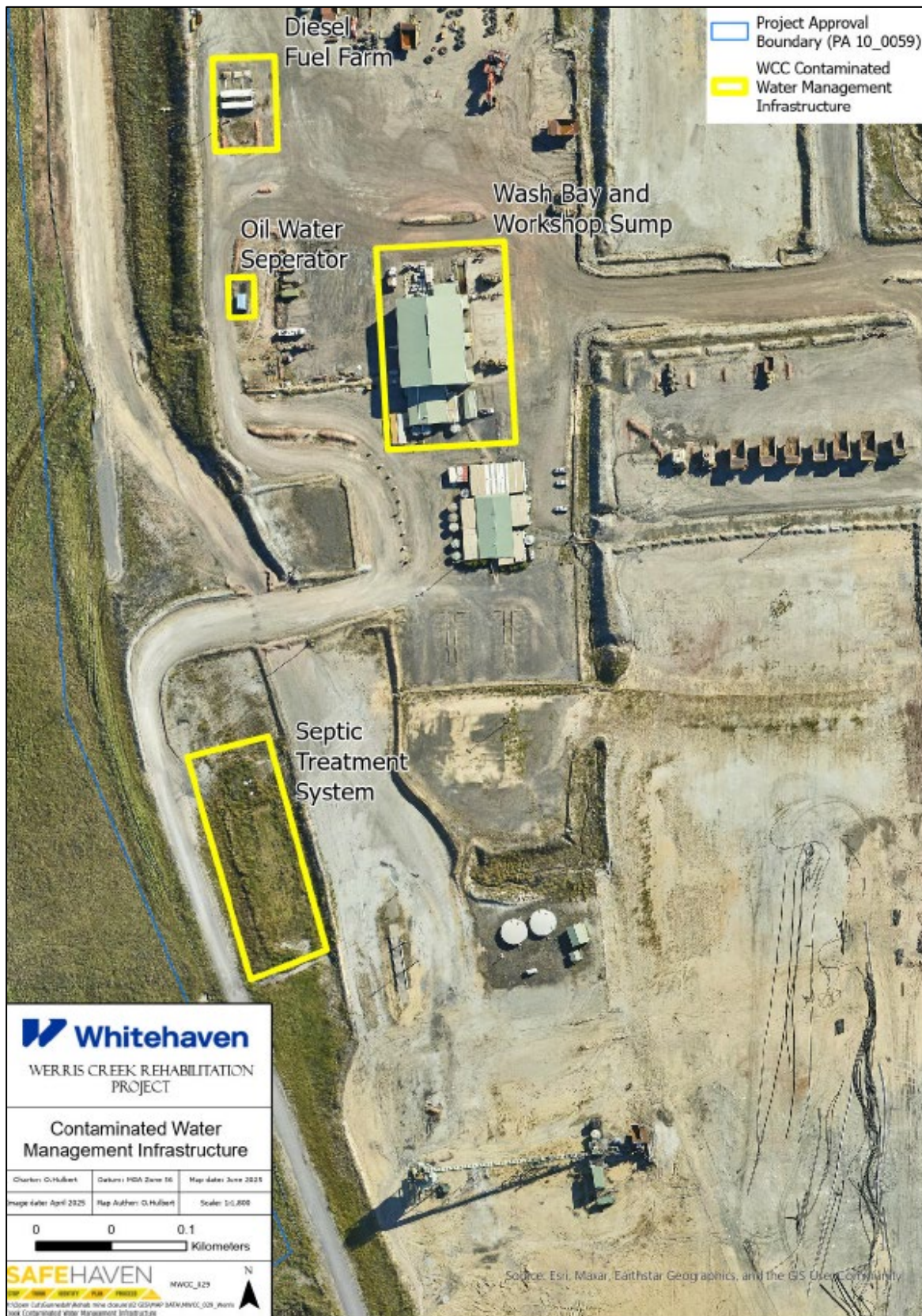
Figure 19 - Contaminated Water Management Infrastructure
