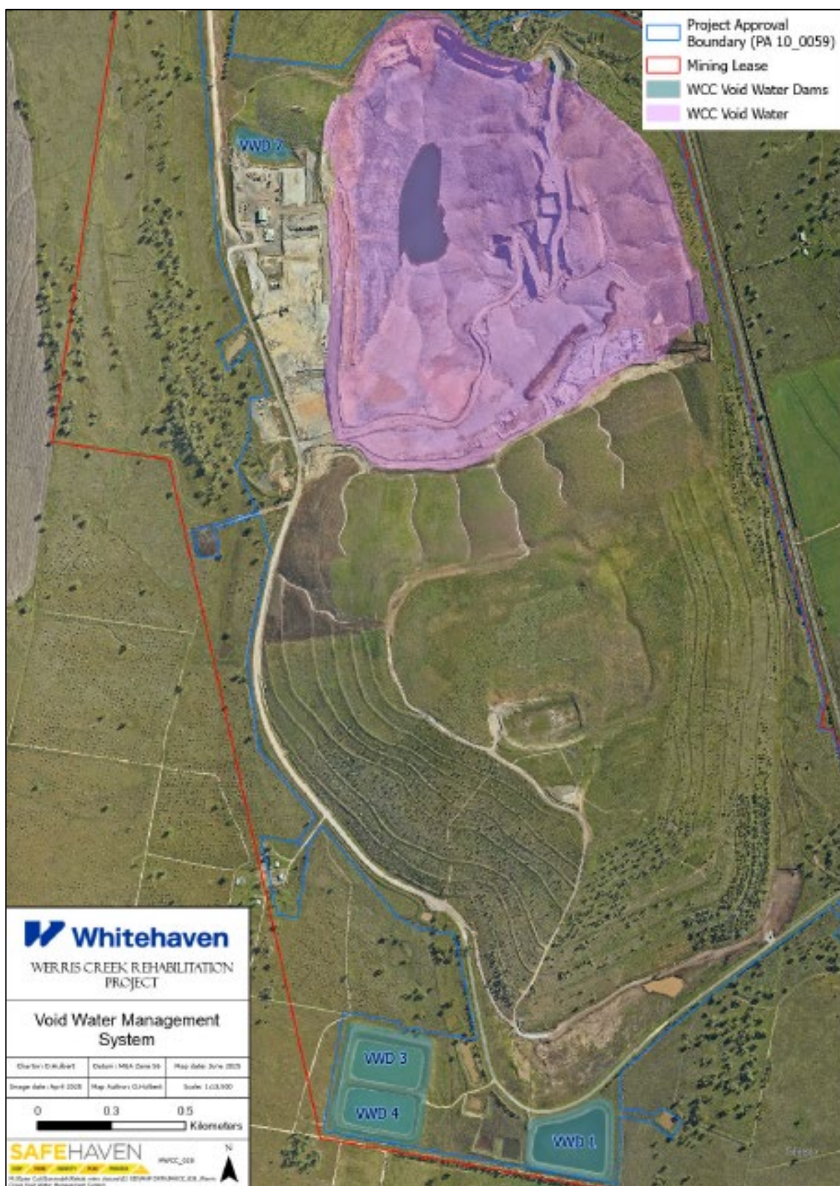
Figure 13 - WCC Void Water Management System
