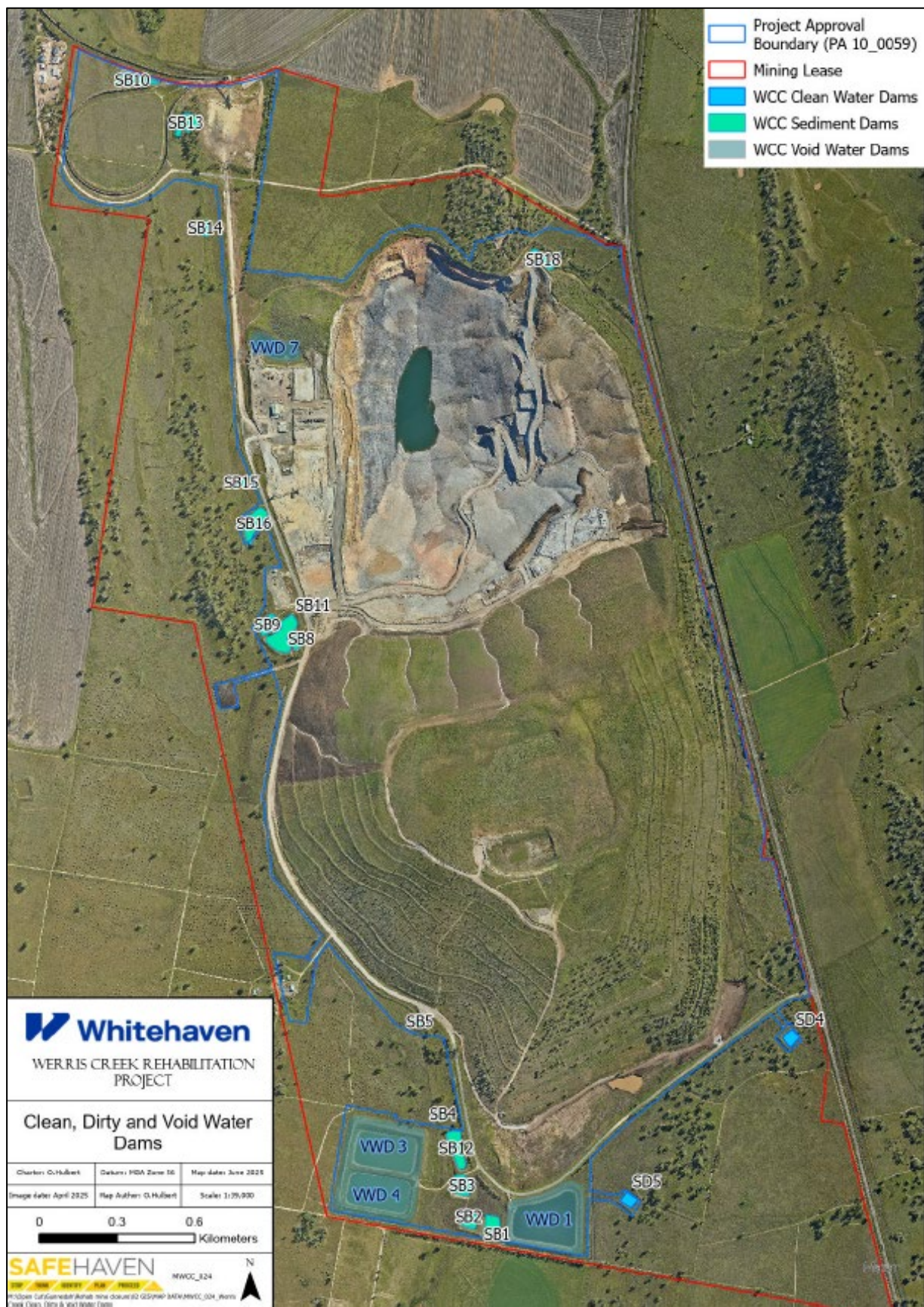
Figure 20 - Clean, Dirty and Void Water Dams Onsite at WCC
